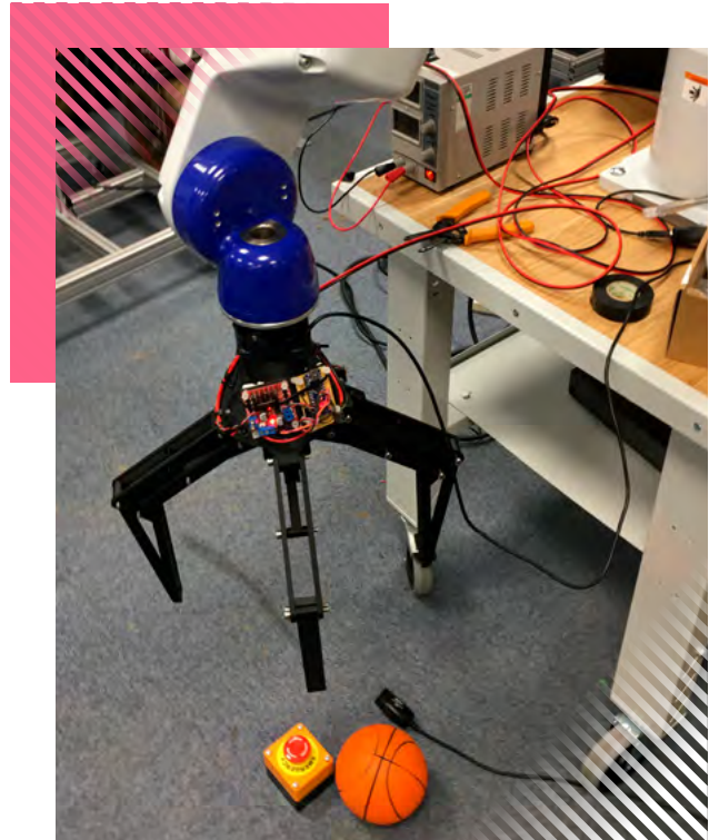
Robot with gripping end of arm tools using computer vision to grasp objects (Research & Innovation Festival 2020, University of Plymouth)
